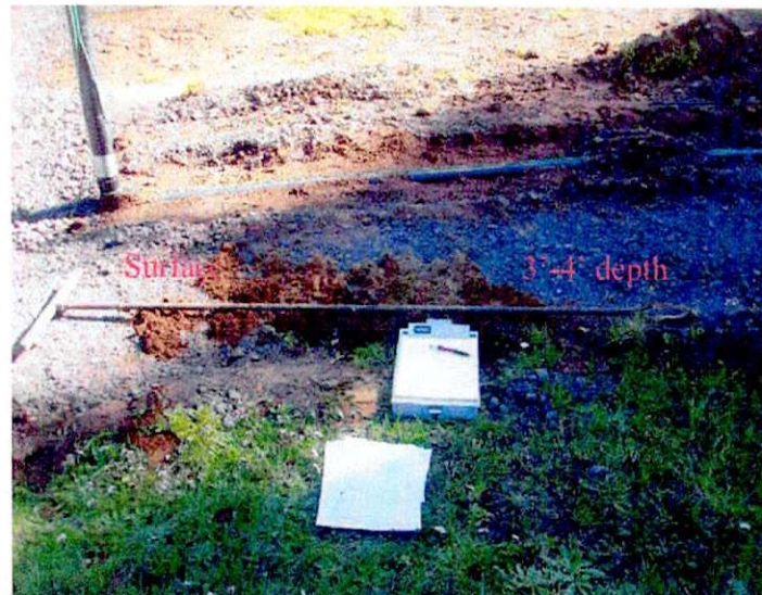
HA1 soil cuttings, which were loose to somewhat dense, fine-sandy silt at the surface to very loose fine to medium sand at 3-4 feet bgs.
