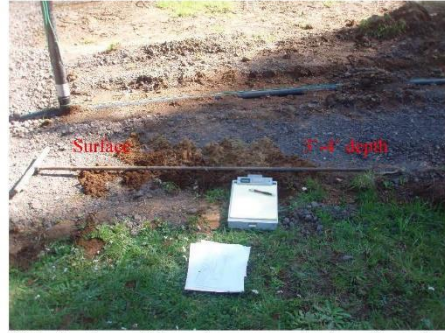
HA1 soil cuttings, which were loose to somewhat dense, fine-sandy silt at the surface to very loose fine to medium sand at 3-4 feet bgs.
