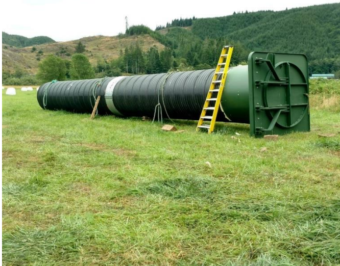
Figure 3. Typical side-hinged aluminum tidegate mounted on 6.0ft CMP.
