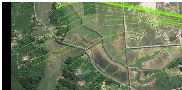
Figure 2. Plan view of hydraulic model layout showing cross-section locations. Figure is oriented with North to the top and water flow from right to left on figure.
