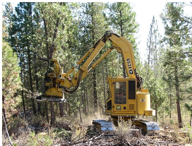
A feller-buncher is a common piece of equipment used for mechanical treatments. Photo credit: Oregon Department of Forestry.
