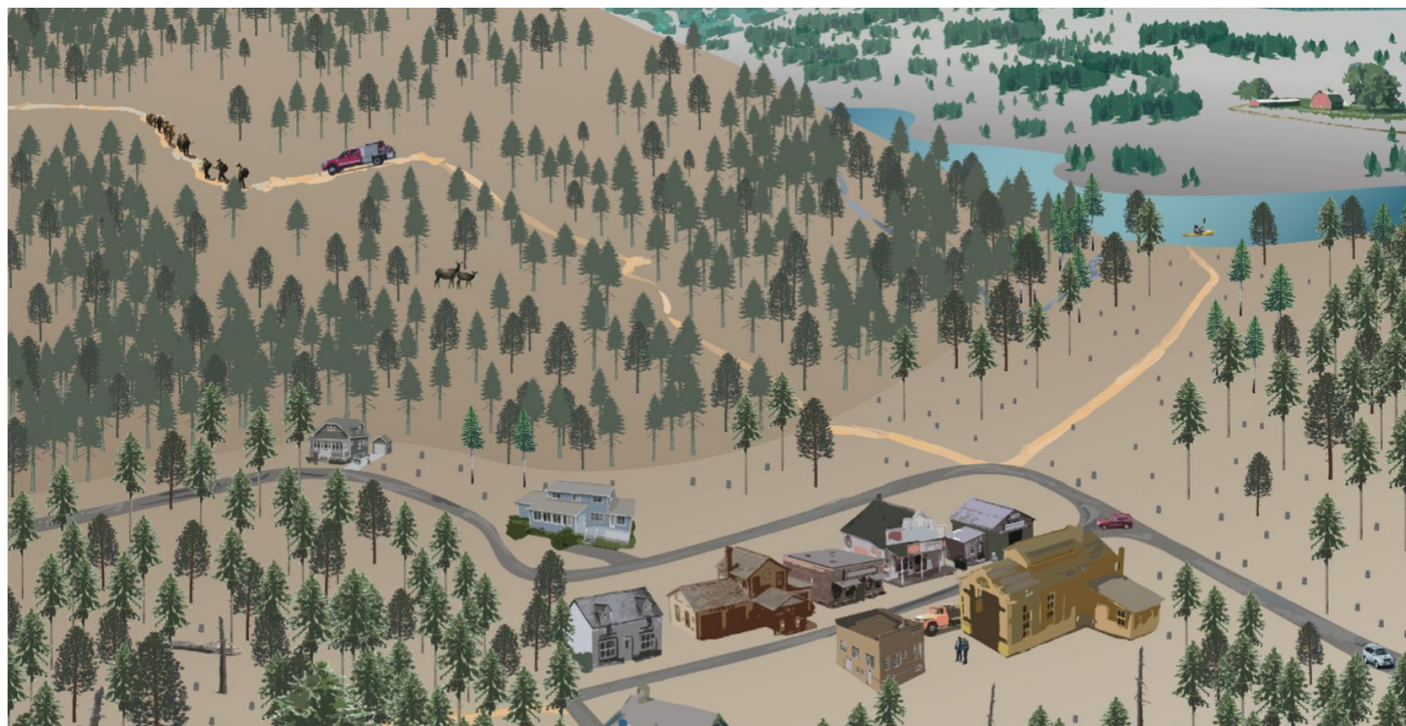
Figure 4.c.1. Fuel breaks along roadsides can enhance the ability of firefighters to use roads as potential control lines for fire suppression and proactive management of fire on the landscape, and they can make roads safer for residents during evacuations. Source: WA DNR (Hersey and Barros, 2022).
