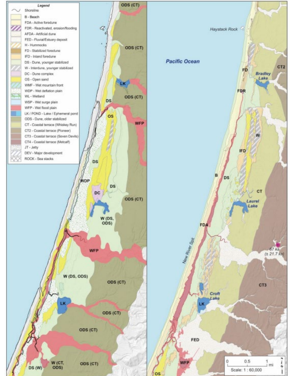
Figure 4.3. Beach and dune geomorphic mapping classifications for the New River Spit. (left) original USDA (1975), (right) updated version. Green and pink circles, respectively, denote 14 C and thermoluminescence (TL) dates determined by Peterson and others (2007).
