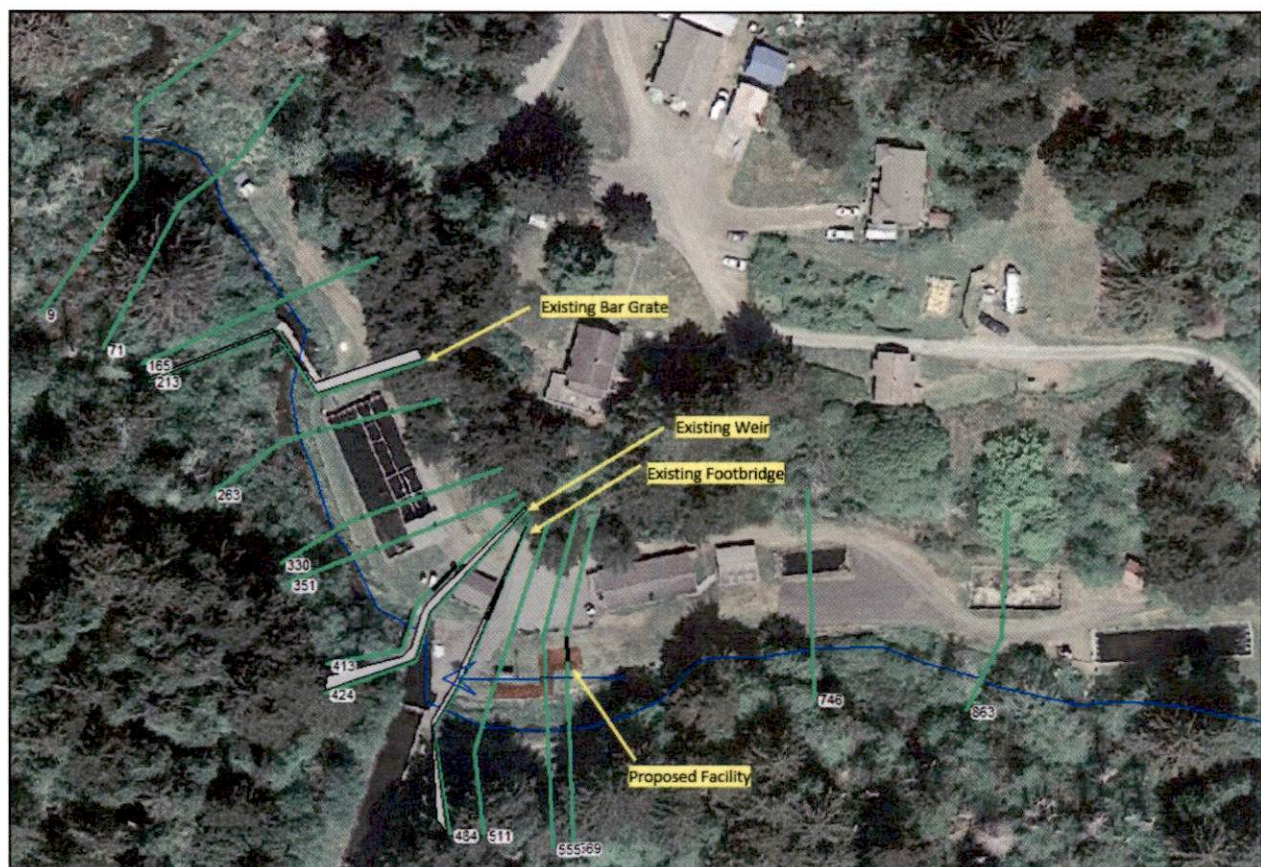
Figure 4. Plan view of hydraulic model geometry showing cross-section locations (green), Ferry Creek centerline (blue), existing infrastructure (grey), existing buildings, and proposed Restroom Facility boundary (red), overlain on aerial map. Water flows from right to left on the figure.
